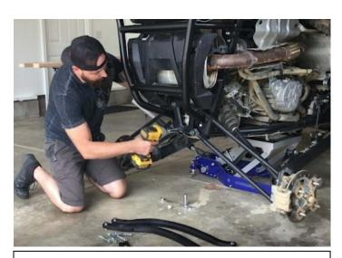
Remove the OEM rear lower radius rods by removing the existing bolts at the frame and spindles using an impact with an 18mm socket and an 18mm wrench.
