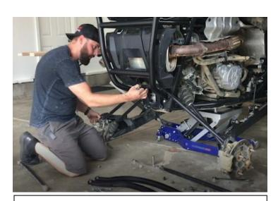
Remove the upper radius rod only at the frame, leave the upper radius rod attached to the spindle. Next you will remove the plate.
