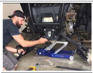
Position the radius rod in between the plate and the spacer, and slide the provided flange bolt into place. Secure it with the provided nyloc nut. Repeat on the other side.
