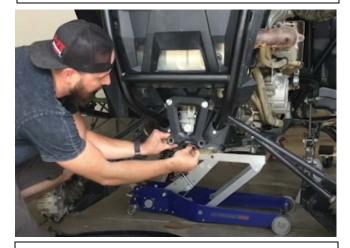
Insert the "U" shaped spacer bracket in between the frame and the plate. The flat part should be facing down, making it appear as a "U" if installed
