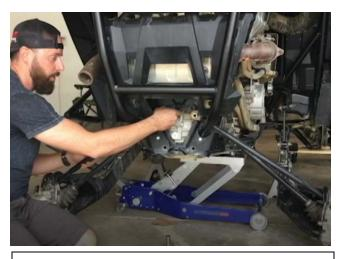
Take the straight spacer bracket and place it in between the frame and upper radius rods and the mounting point.
