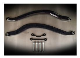
Warning: If you have a 2016 and older unit, using a 12mm drill bit you will need to drill out the lower radius rod mounts at the frame, lower mounts on the radius rod plate, and the lower mount on the spindles in order to use these radius rods.
