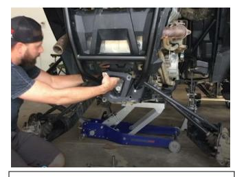
Reattach the plate using two of the provided flange bolts and nylon lock nuts at the upper two mounts, securing the upper radius rods with the bracket. (For 2016 and older models, use the M10 x 1.75 x 80)
